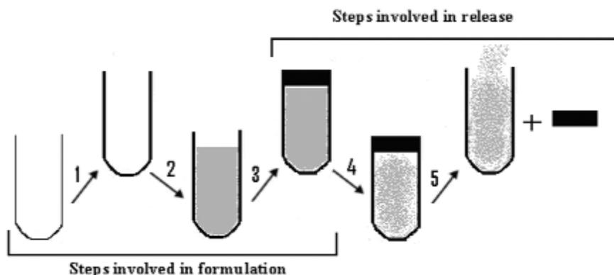
**Figure 1.** Key steps in formulation and release of acetaminophen osmotic capsular system: (1) semipermeable coating; (2) ingredients filling; (3) placement of plug; (4) simultaneous build up of osmotic and hydrostatic pressures inside the capsule due to water penetration from the sink; and (5) start of drug release after plug expulsion.
