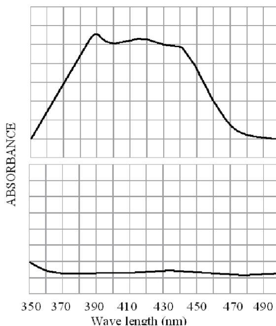
**Figure 1.** Absorption spectra of the ethyl maltol-Fe(III) complex (A) against reagent blank (B). The concentration of Fe(III) was kept at  $5 \times 10^{-5}$  M. pH=5, ethyl maltol:Fe(III) molar ratio=1:10, t = 2.5 h.
