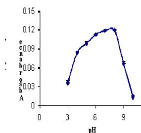
**Figure 2.** The effect of pH on the absorbance of ethyl maltol-Fe(III) complex. The concentration of Fe(III) was kept at  $5 \times 10^{-5}$  M, Ethyl maltol:Fe(III) molar ratio=1:10,  $t=2.5$  h,  $\lambda=395$  nm. Each data point plotted represents the mean absorbance value for nine replicate absorbance readings. Error bars represent the standard deviation between consecutive measurements of each sample.
