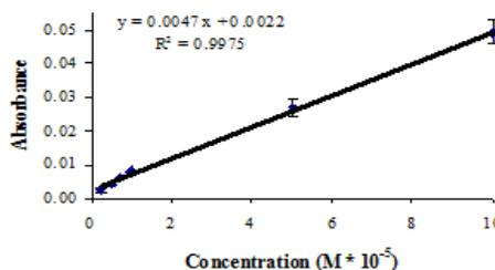
**Figure 6.** Standard curve for the determination of iron(III) with atomic absorption spectrometry. Each data point plotted represents the mean absorbance value at 248.3 nm for six replicate absorbance readings. Error bars represent the standard deviation between consecutive measurements of each sample.
