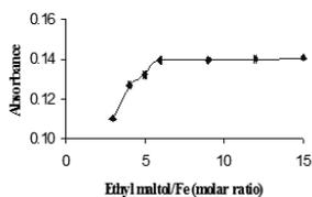
**Figure 4.** The effect of increasing ratio of ethyl maltol to Fe(III) on the absorbance of the ethyl maltol-Fe(III) complex. The concentration of Fe(III) was kept at  $7.5 \times 10^{-6}$  M. pH=7, t=2.5 h,  $\lambda=395$  nm. Each data point plotted represents the mean absorbance value for nine replicate absorbance readings. Error bars represent the standard deviation between consecutive measurements of each sample.
