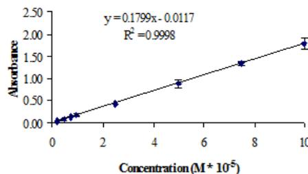
**Figure 5.** Standard curve for the determination of iron(III) with ethyl maltol-Fe(III) complex formation. pH=7, ethyl maltol:Fe(III) molar ratio=1:10, t = 2.5 h,  $\lambda=395$  nm. Each data point plotted represents the mean absorbance value at 395 nm for six replicate absorbance readings. Error bars represent the standard deviation between consecutive measurements of each sample.
