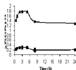
**Figure 3.** The effect of time on ethyl maltol-Fe(III) complex formation. The concentration of Fe(III) was kept at  $2.5 \times 10^{-5}$  M (square) or  $1 \times 10^{-4}$  M (triangle). pH=7, ethyl maltol:Fe(III) molar ratio=1:10,  $\lambda=395$  nm. Each data point plotted represents the mean absorbance value for nine replicate absorbance readings. Error bars represent the standard deviation between consecutive measurements of each sample.
