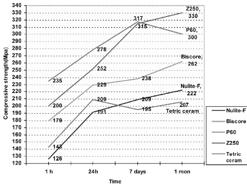
**Figure 1.** Mean compressive strength of composite resins in different times.
