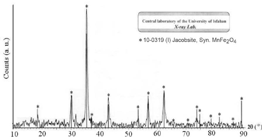
Figure 1. XRD pattern of the coprecipitated Mn ferrite.
