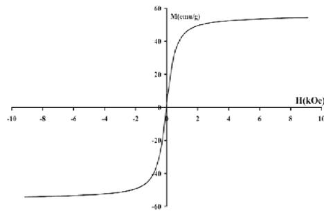
**Figure 3.** Room temperature hysteresis loop of the coprecipitated Mn ferrite.
