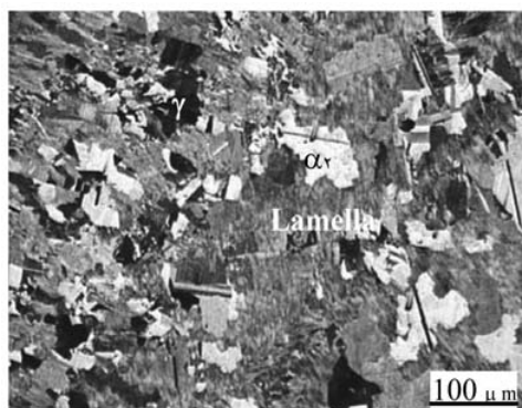
Figure 1. Microstructure of Ti-47Al-2Cr after homogenizing.
