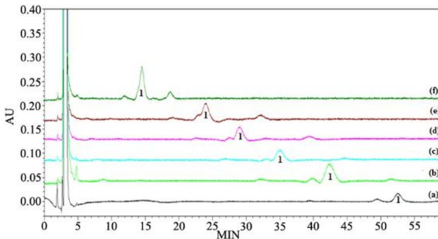
**Figure 3.** Chromatogram of (1) eluted with isocratic mobile phase of a) 88% b) 89%; c) 90%; d) 91%; e) 92%; f) 95% of methanol in water.
