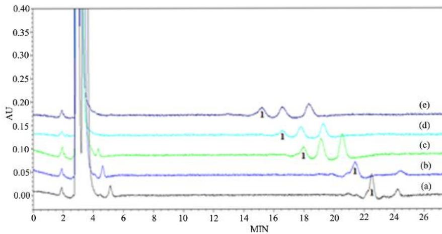
**Figure 2.** Chromatogram of (1) eluted with a gradient mobile phase consisted of a) 87–100%; b) 90–100%; c) 92–100%; d) 93–100%; e) 94–100% methanol and water.
