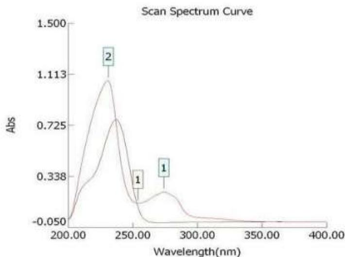
**Figure 3.** Overlay spectrum of dolutegravir and rilpivirine.
