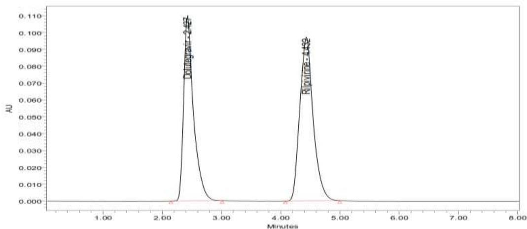
**Figure 4.** Chromatogram showing specificity of dolutegravir and rilpivirine.
