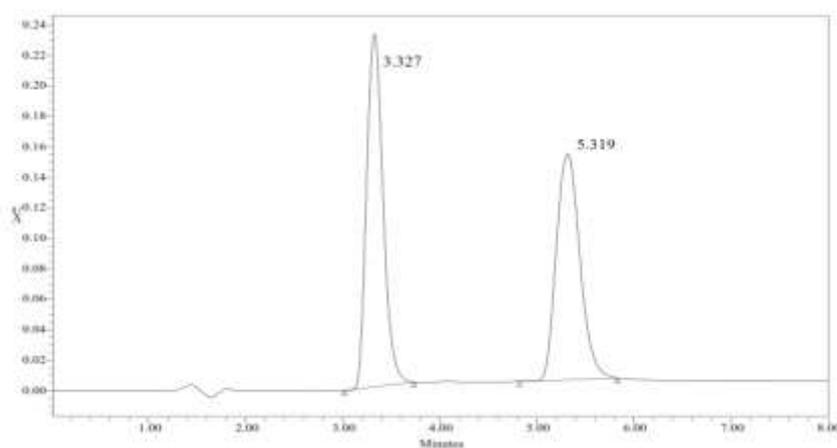
**Figure 11.** Chromatogram showing robustness solution of decreased mobile phase flowrate (0.6 ml/min) of dolutegravir and rilpivirine.
