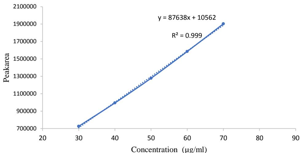
**Figure 6.** The Linearity curve of (30-70 µg/ml) rilpivirine.
